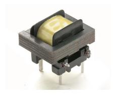
This PC mount current transformer is a low-cost solution – it is used in a frozen drink machine to ensure proper consistency of finished product. Rather than measure temperature of processed drink mixture, Standex-Meder engineers suggested measuring current draw – providing a more consistent end product.
