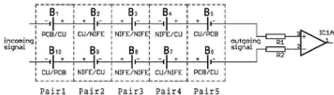
Figure 1. Two pole Reed Relay thermocouple schematic.
