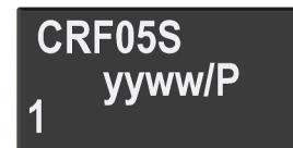
Marking according to EN60062/factory code gem. EN60062/Fertigungsstätte
